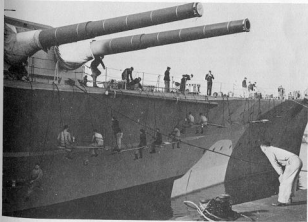
The dark color on the Bismarck 's gun barrels is red lead. It was normally applied when the barrels' gray paint blistered and peeled from the heat of extensive firing and had to be scraped. The rings around the guns hold a cable connecting a coil (visible at the muzzle) to an instrument in the turret which measures each shell's time of flight. (Photograph from Ferdinand Urbahns.)
