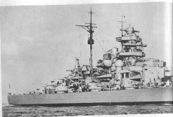
The Bismarck shows her rakish, modern lines in Kiel Bay in late 1940. A censor slightly altered her appearance by removing the radar antenna from her foretop range-finder cupola. (Photograph courtesy of Blohm & Voss.)
